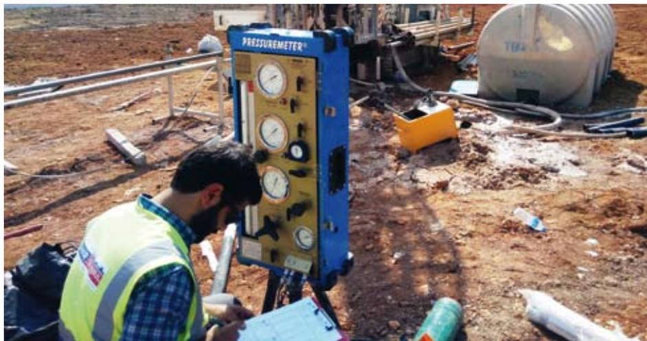
Trevi is involved in the soil investigations site for the new line of the Istanbul underground "Bostancı - Dudullu Metro Line". The geotechnical campaign, carried out on behalf of Geodata Italia S.p.A, consists in core drilling works, on-site tests (pressuremeter, dilatometer, water tests) and laboratory tests.
