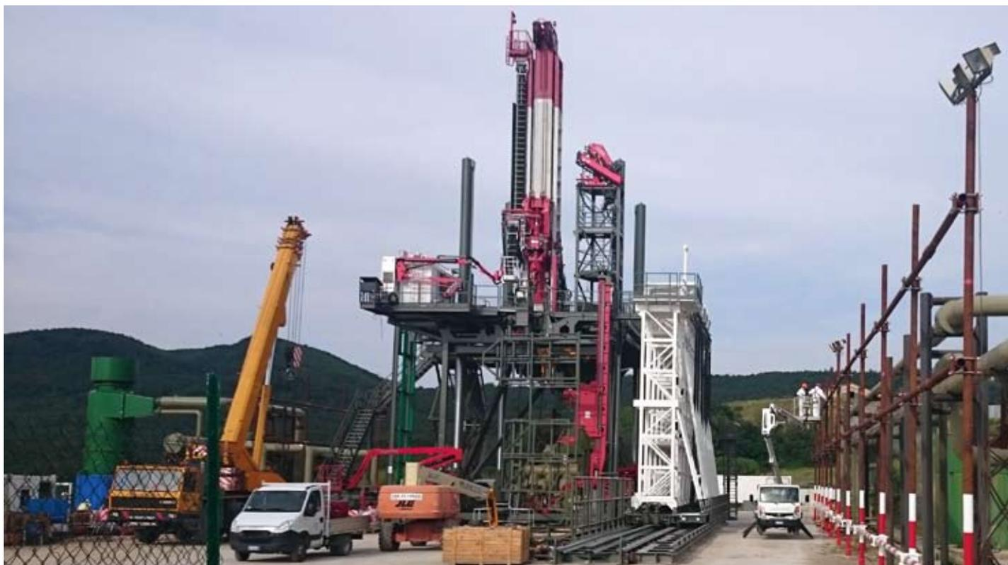
The end of the commissioning was celebrated with an event which saw the presence of leaders from both Enel and Drillmec at the yard located in Castel Nuovo Val di Cecina, province of Pisa (Italy). The HH-300 (second rig supplied to EGP) allows to overcome the operating limits of conventional drilling systems in the geothermal sector, such as the handling system of the drill
